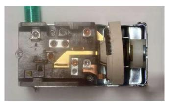
**NOTE 1:** If you are using this new AAW switch in a **1953-55 Ford Truck** that originally used a 6 volt switch, you will find that the threaded area on your original nut is too small in diameter. You will need to purchase a new 1956 12 volt style replacement nut which is larger in diameter and will fit this new AAW switch and still allow for the use of your stock dash bezel. These are readilly available from your favorite truck parts supplier.
